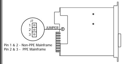
Anti-Arcing Protection: Jumper J7 is to prevent damage to the contact points of the controller when removed from the mainframe while power is still on. J7 is set to pins 2 & 3 by factory default. If the controller is placed in a non-PPE mainframe, place jumper on pins 1 & 2. If jumper is placed incorrectly, a TOH error may occur (NO POWER OUPUT).
